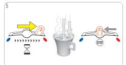
Push selection lever to the "HOT" or "COLD" position as recommended on capsule packs. Beverage preparation starts. Wait until the lever moves to the "STOP" position. Extraction stops. Extraction can be stopped manually by moving the lever back to the "STOP" position.
