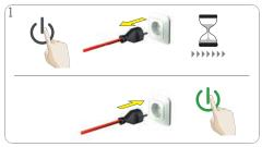
Switch off machine. Check if capsule is blocked, see 9.2 "NO LIQUID COMES OUT — CAPSULE / INJECTOR BLOCKED?" on page 15. Unplug power plug and wait 20 minutes. Afterwards plug power plug into mains power socket and switch machine on.
