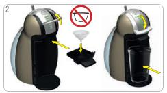
Open locking handle. Make sure that rinsing tool is in capsule holder and capsule holder is in machine. Close locking handle. Place an empty large container underneath the coffee outlet.
