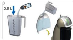
Mix 0.5 liter fresh drinking water with descaler in a measuring cup. Pour descaling solution into water tank and insert water tank into machine.
