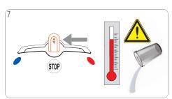
Wait until the lever moves to the "STOP" position. Extraction stops. Empty and clean container. Waming: Hot water! Handle with care!
