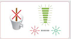
No liquid comes out: Beverage preparation stops part way during delivery or does not start at all. Bar display flashes and power button blinks red and green rapidly.
