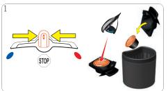
Push selection lever to the "STOP" position. Pull out capsule holder. Put used capsule in capsule bin.
