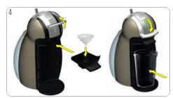
Open locking handle. Put rinsing tool into capsule holder. Insert capsule holder into machine. Close locking handle. Place an empty large container underneath the coffee outlet.
