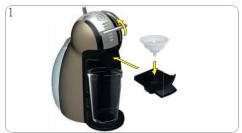
Put rinsing tool into capsule holder. Insert capsule holder into machine.
