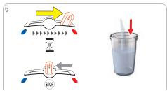
Push selection lever to the "HOT" position. Machine descales in start-stop operation for approximately 2 minutes. Lever comes back to the middle position.
