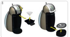
Open locking handle. Pull out capsule holder. Remove rinsing tool. Place drip grid on drip tray. Then insert drip tray at desired position. If any, remove water from water tank.
