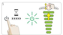
Press and hold power button for at least 5 seconds. Power button blinks green. Machine enters descaling mode. Set bar display to maximum level with selection lever.
