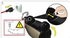
Unplug power plug! Remove drip grid and drip tray. For better access to injector tilt machine. Never touch injector with finger! Clean injector with cleaning needle. Follow instructions in 8. "Descaling at least every 3-4 months" on page 13.
