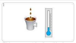
If the beverage comes out slower than usual (even in droplets), or if it is cooler than usual the machine has to be descaled.
