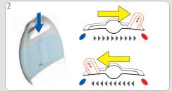
Check if the water tank contains enough fresh drinking water. If not, refill with fresh drinking water and push selection lever to the "HOT" position respectively "COLD" to continue preparation. If the water tank is full proceed as described in 9.2 "NO LIQUID COMES OUT — CAPSULE / INJECTOR BLOCKED?" on page 15.
