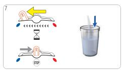
Push selection lever to the "COLD" position. Machine descales continuously. Lever comes back to the middle position.
