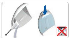
Rinse and clean water tank. Use a clean food-safe brush and washing-up liquid as needed. Afterwards refill with fresh drinking water and insert it into machine. The water tank is not dishwasher proof!
