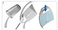
Empty and clean container. Rinse and clean water tank. Use a clean food-safe brush and washing-up liquid as needed. Afterwards refill with fresh drinking water and insert it into machine.
