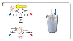
Push selection lever to the "COLD" position. Wait until the lever moves to the "STOP" position. Extraction stops.
