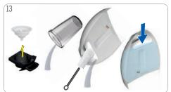
Pull out capsule holder. Remove rinsing tool. Rinse capsule holder with fresh drinking water from both sides. Reinsert capsule holder. Empty and clean container. Rinse and clean water tank. Afterwards refill with fresh drinking water and insert it into machine.
